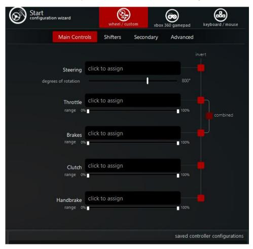
Click the axis you would like to assign, afterwards you should actuate the given input, so for steering rotate the steering wheel and so on.
